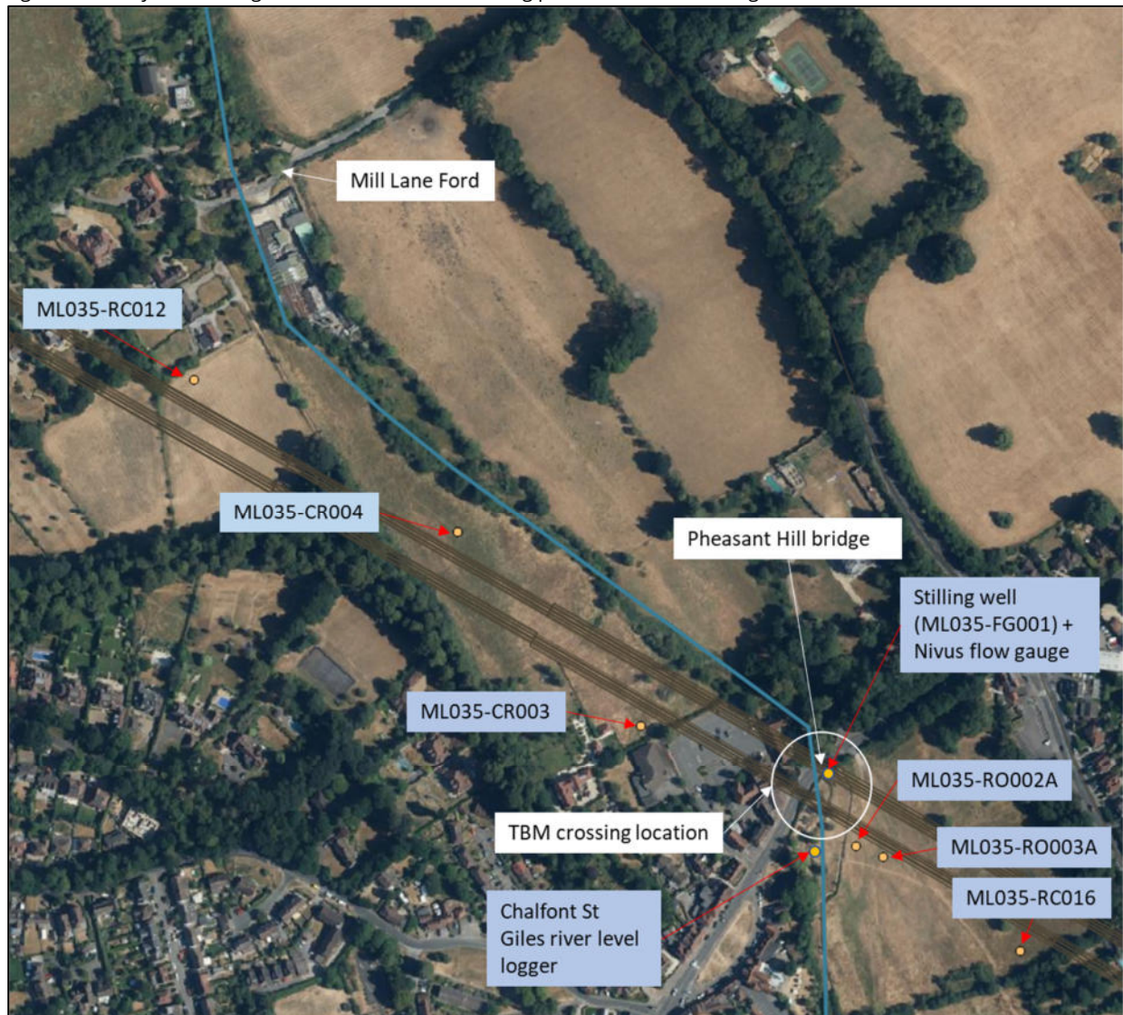
Figure 3: Site layout showing locations of water monitoring points and TBM crossing location
